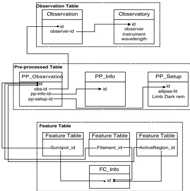
Figure 2. The SFC database structure: the observation, pre-processing and feature tables.
