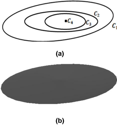
**Figure 4. An example wound surface generated by the fourth order PDE where the conditions are all taken to be function conditions. (a) The conditions defined in the form of curves in 3-space. (b) The resulting wound surface shape.**
