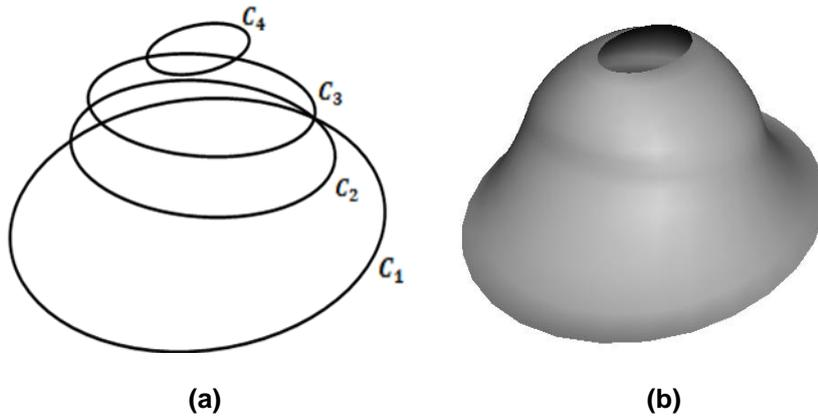
**Figure 2. The shape of a surface generated by the fourth order PDE where the conditions are all taken to be function conditions. (a) The conditions defined in the form of curves in 3-space. (b) The resulting surface shape.**
