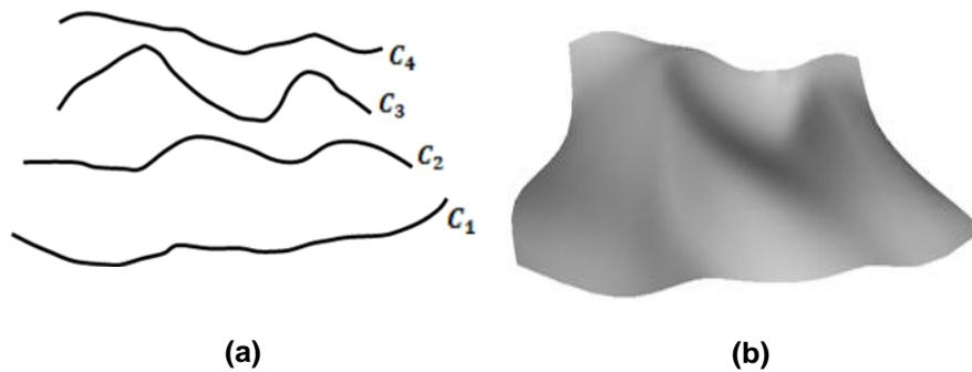
**Figure 3. A four-sided surface patch generated by the fourth order PDE where the conditions are all taken to be function conditions. (a) The conditions defined in the form of curves in 3-space. (b) The resulting surface shape.**
